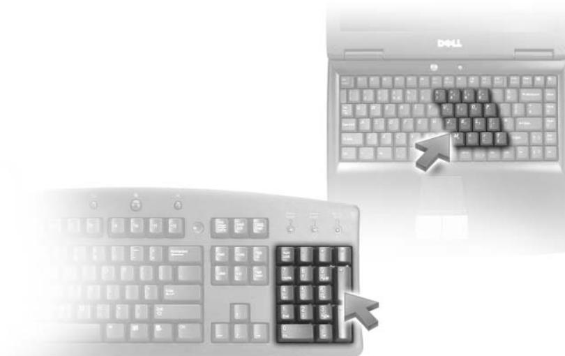
The numeric keypad functions like the numeric keypad on an external keyboard. Each key on the keypad has multiple functions. The keypad numbers and symbols are marked in blue on the right of the keypad keys. To type a number or symbol, press <Fn> and the desired key after enabling the keypad.
