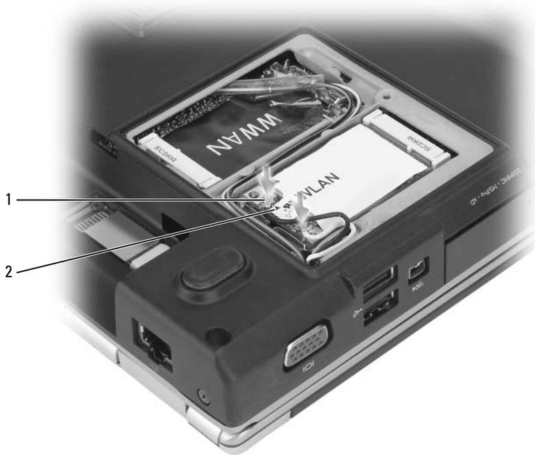
1 antenna cable connectors (2) 2 triangles (2)
